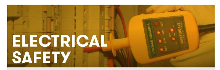
Any engineer working on a piece of electrical equipment or supply circuits needs to ensure supplies are isolated and locked off in such a way to avoid risk of electrocution by accidental energisation. Equipment also needs to be tested to ensure no risk to users, including testing circuits and machinery earthing, insulation, and to ensure all portable appliances are damage-free.
