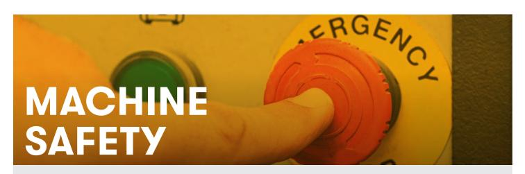
Virtually all industrial machinery posses potential risks. The European Machinery Directive 2006/42/EC defines they be assessed and steps taken to mitigate them. This mitigation can include physical guarding, but also machinery safety products which act as electrically controlled safe guards reducing the risk of injury.
